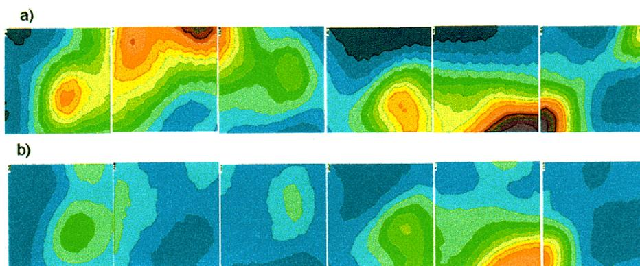
**Figure 14.** The map of the same strip (dimensions 1 cm by 6 cm). (a) In the central part of the sheet, 25 cm by 25 cm; (b) after cutting the sheet into 3 cm wide strips and annealing.
