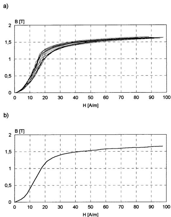
**Figure 7.** Comparison of the toroid steel sample investigations. (a) Magnetizing curve for  $H$  determined by remote sensors in 16 randomly selected points; (b) magnetizing curve for  $H$  determined from magnetizing current.
