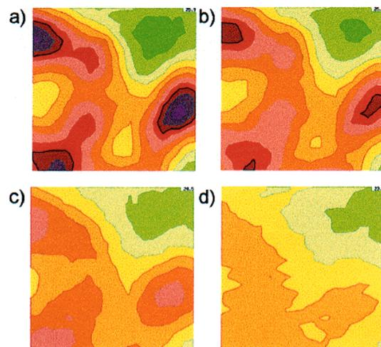
Figure 3. The maps of magnetic field for various distances between the sensor and the sheet surface. (a) 0.3 mm, (b) 0.5 mm, (c) 1 mm and (d) 2 mm.
