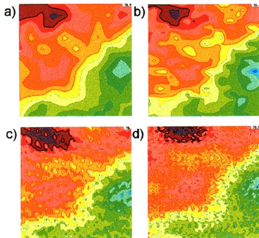
**Figure 4.** The maps of field distribution for various measurement points densities. (a) 1 mm, (b) 0.5 mm, (c) 0.25 mm, and (d) 0.125 mm.
