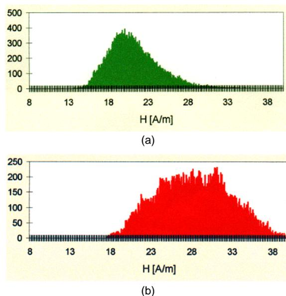
**Figure 10.** The histograms of magnetic field strength distribution above two different sheets. (a)  $P_1 = 0.35 \text{ W kg}^{-1}$ , (b)  $P_1 = 0.51 \text{ W kg}^{-1}$ .
