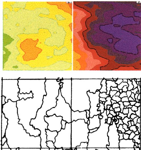
**Figure 11.** The grain structure of a sheet with corresponding magnetovision map.
