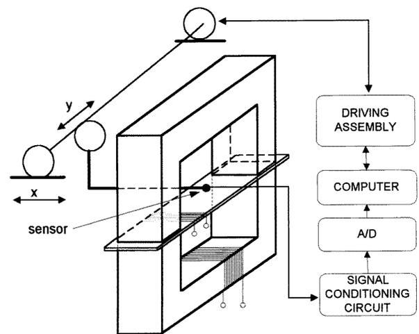
Figure 1. The principle of magnetovision system operation.
