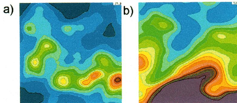
**Figure 15.** Materials deterioration after cutting with poor quality cutting device: the same sheet area before (a) and after (b) cutting into the strips.
