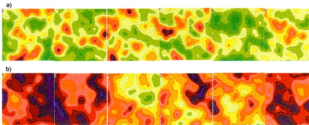
**Figure 9.** The maps of two stripes (dimensions 18 cm by 3 cm) with different specific loss measured by the Epstein method. (a)  $P_1 = 0.35 \text{ W kg}^{-1}$ , and (b)  $P_1 = 0.45 \text{ W kg}^{-1}$ .
