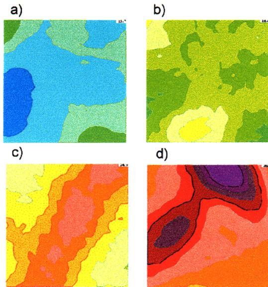
**Figure 8.** The maps of four materials with different power loss. (a)  $P_1 = 0.31 \text{ W kg}^{-1}$ , (b)  $P_1 = 0.37 \text{ W kg}^{-1}$ , (c)  $P_1 = 0.45 \text{ W kg}^{-1}$ , and (d)  $P_1 = 0.51 \text{ W kg}^{-1}$ .
