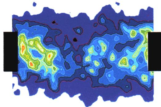
Figure 2. The map of magnetic field distribution for a sheet placed over the yoke. The yoke poles dimensions are 3 cm by 2.5 cm, and they are situated 8 cm apart.
